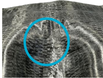
Bridging, In-plane / Out-of-plane wrinkles
