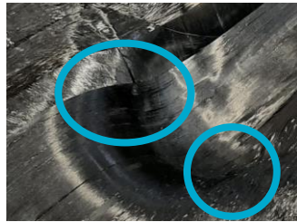
Tape folding, Gapping, Wrinkles, Fibre Orientation
