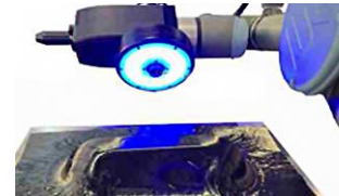
Optical Inspection (Top Layer) In-plane wrinkles, Tape folding, Gapping, Fibre Orientation
