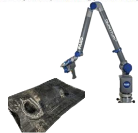
Laser Scanning Arm Bridging, Out-of-plane wrinkles, Tape folding, Gapping
