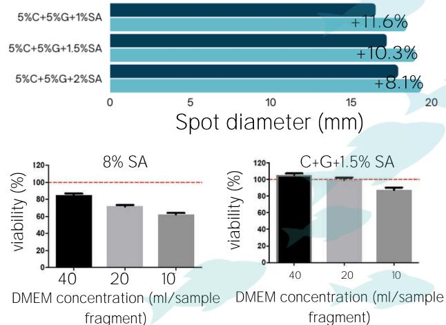
The addition of sodium alginate to the collagen and gelatine foams increases the open porosity of the sample. However, as the sodium alginate concentration increases, this parameter decreases slightly. The wettability test also confirms this. Furthermore, the rheological test confirms that an excessive alginate concentration in the solution negatively affects its rheostability.
