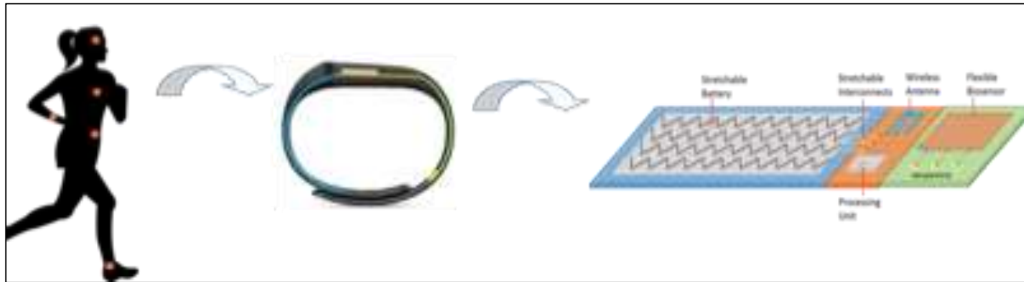
body conformable electronic bracelet with biological sensors powered by the stretchable microbattery
