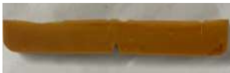
Heated cured DGEBA/HydDA at 140°C
