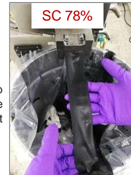
Electrode strip recovered at the extruder outlet
